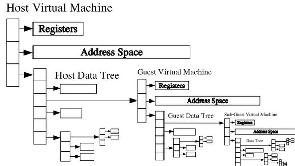
only stored once in memory or on disk (copy-on-write optimization), allowing hosts to store snapshots of guest computations efficiently at any desired frequency.
